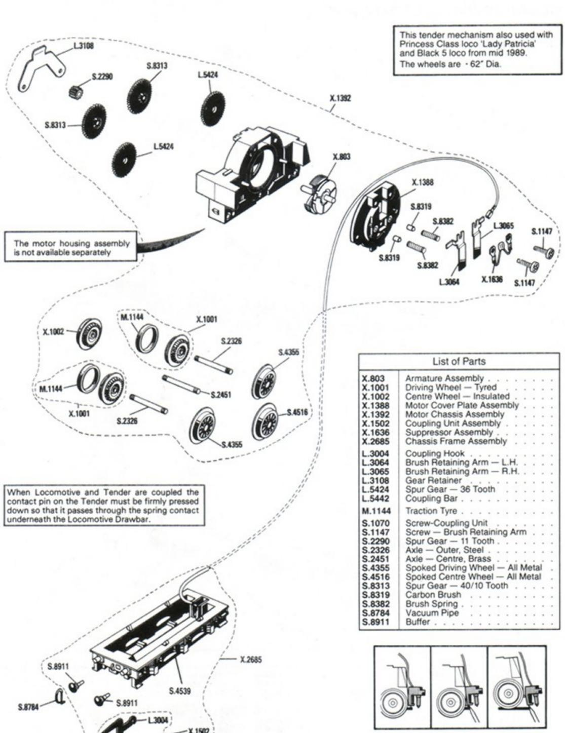
(X.1392), prise Coupling Pin forward with a small screwdriver, then press Motor Chassis Assembly out of the Chassis Frame. The Coupling Pin (shaded) cannot be removed from the
